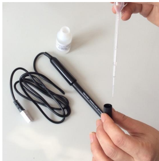
Picture 23: Filling the electrode membrane cap
