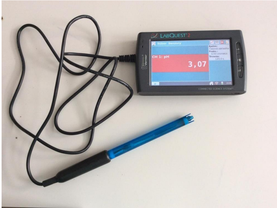
Picture 3: Example of Sensor Connection to the Measurement Interface Unit
