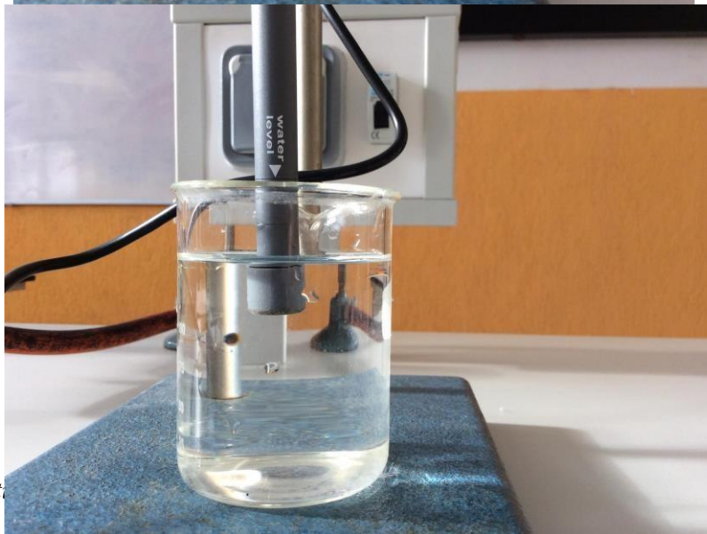
Picture 15: Correct submersion of the sensor into the sample
