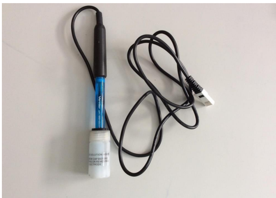
Picture 2: Vernier pH Sensor in Storage Solution
