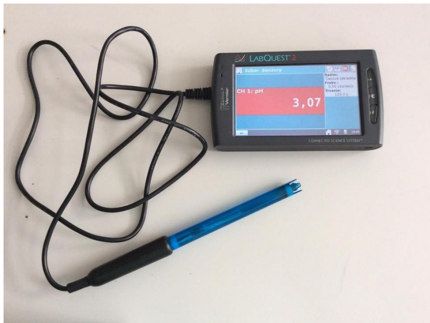
Picture 2: pH Measurement
