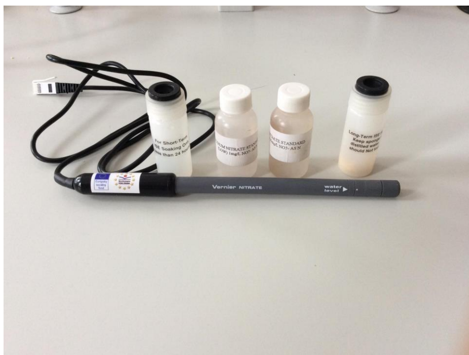
Picture 9: Contents of the nitrate ISE package
