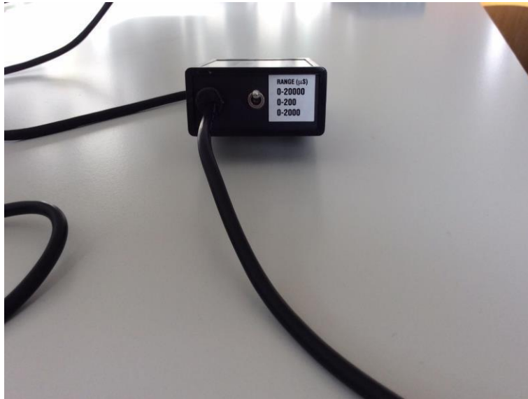
Picture 4: Measurement Range Switch - Use it only during calibration
